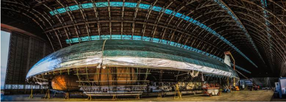
ML806 Dragon Dream was assembled in a World War II-era blimp hangar at the former Marine Corps Air Station in Tustin, CA, which was under license to the Navy. In the above photo, the aeroshell frame and skin on the lower half of the airship are not completely installed, revealing some internal features. Note the rigid aeroshell framing, transverse pressurized helium tanks (orange) and an air expansion volume. Source: Aeros via LinkedIn
