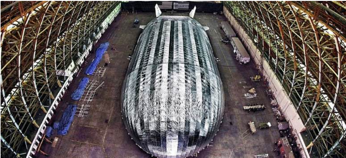
The completed ML806 Dragon Dream with the lightweight skin installed over the rigid aeroshell frame.
