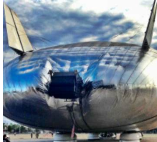
(Above) Stern-mounted, propeller slipstream deflector, side view (L), and stern view with deflector “closed” for up/down thrust deflection (R).
