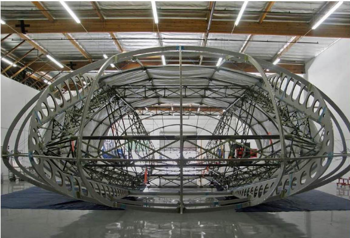
Aeros built this sub-scale Dragon Dream aerostructure under the BAAV program. Source: Aeros
