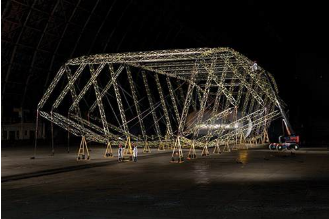
The Dragon Dream's lightweight, rigid main frame, which supports the airship's COSH equipment, its cockpit, cargo, cargo containment structures and aerodynamic control surfaces. Source: Aeros
