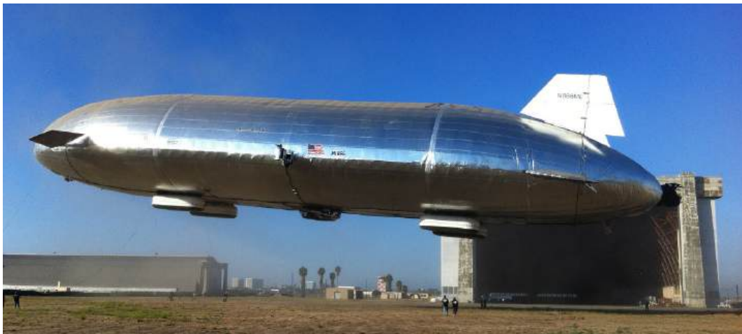
ML806 Dragon Dream flight test, September 2013. The cockpit is visible amidships, under the gas envelope. Source, both photos: Aeros
