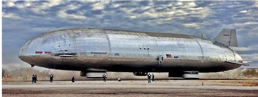
ML806 Dragon Dream outdoor taxi test on its air bearing landing system (ABLS). Source: Aeros (2013)
