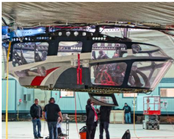
Installation of Dragon Dream cockpit. Source: Aeros
