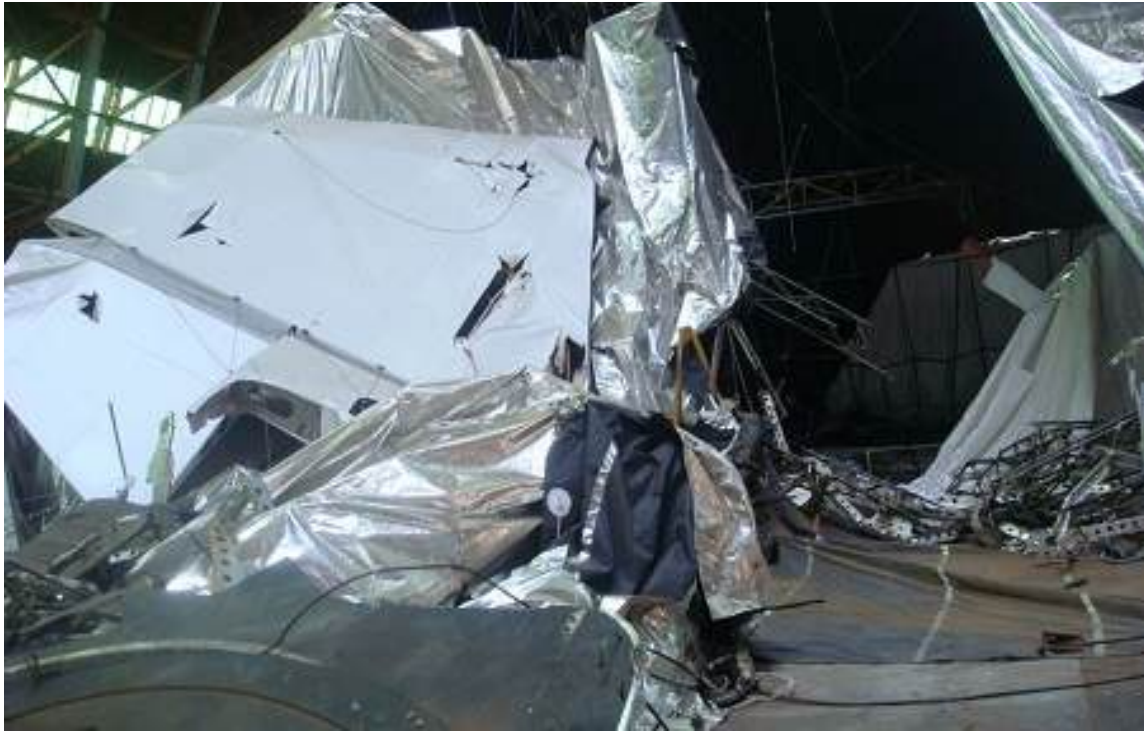
Damage to the rear part of the ML806 Dragon Dream. Source: Allan Ripp via The LTA Society
