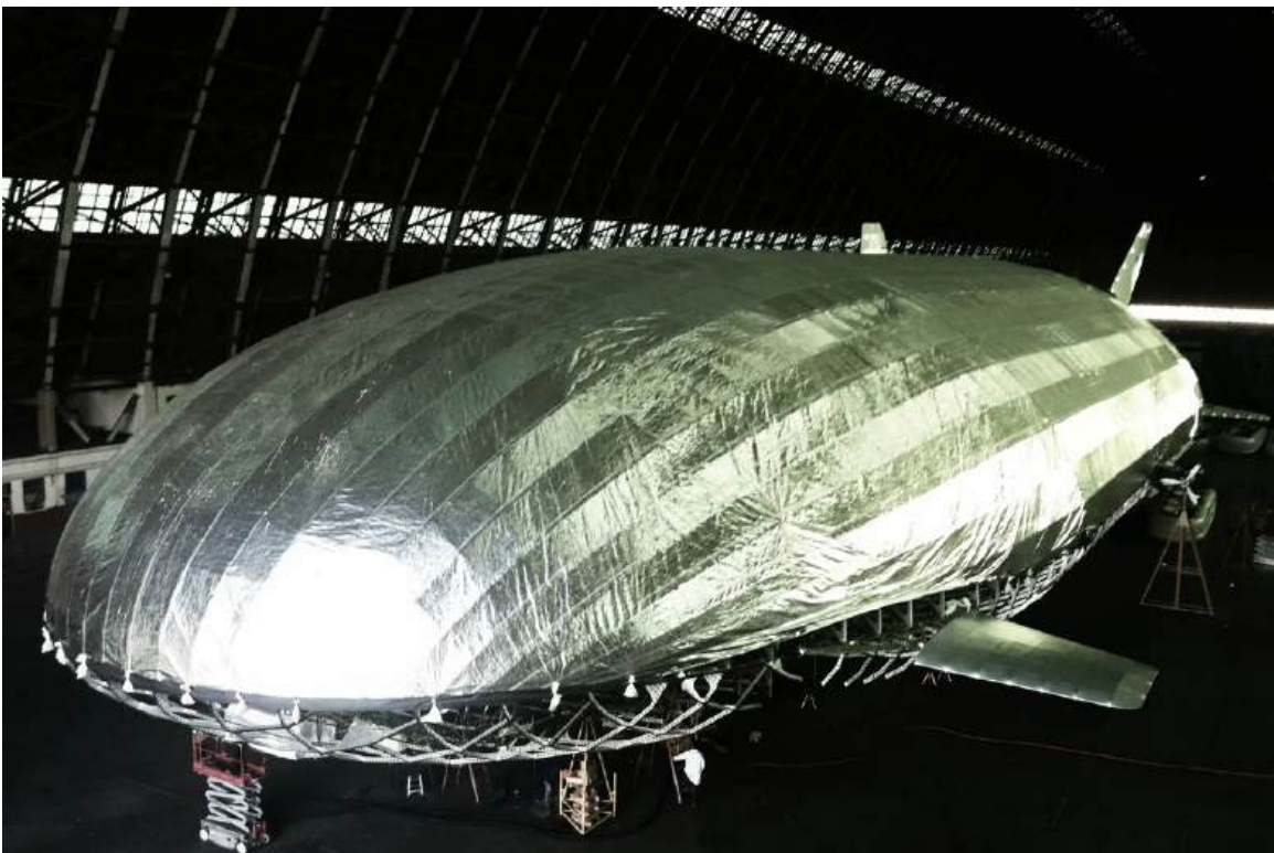
In the above photo, the skin on the lower half of the airship is not installed. Note the attachment of a canard control surface to the rigid aeroshell framing. Source: Aeros
