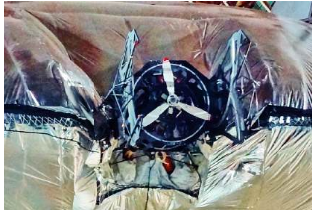
(Above) Flank-mounted thrust-vectoring engine with 3-bladed propeller positioned for cruise (L) and VTOL / hovering (R).
