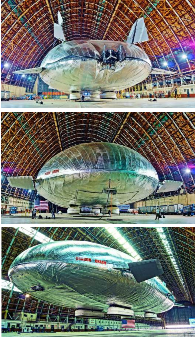
ML806 Dragon Dream's first “static float test” on 3 January 2013. Source: Aeros
