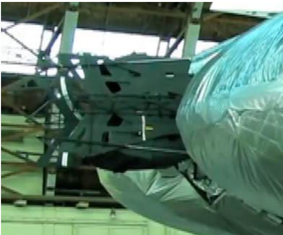
(Above) Stern-mounted, propeller slipstream deflector, side view (L), and stern view with deflector “closed” for up/down thrust deflection (R).
